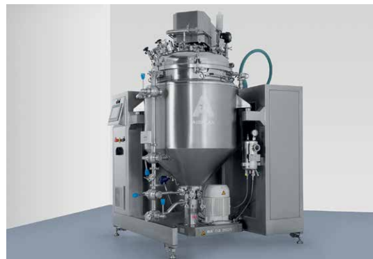
Example of a cream vessel with a bench-mounted temperature control skid
