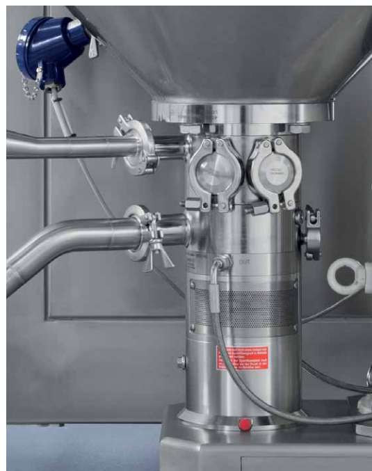
Double mixer system with bottom homogenizing machine and top anchor stirrer with scrapers.
