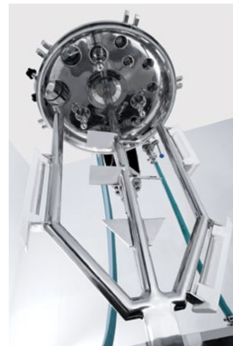
Double mixer system with bottom homogenizing machine and top anchor stirrer with scrapers.
