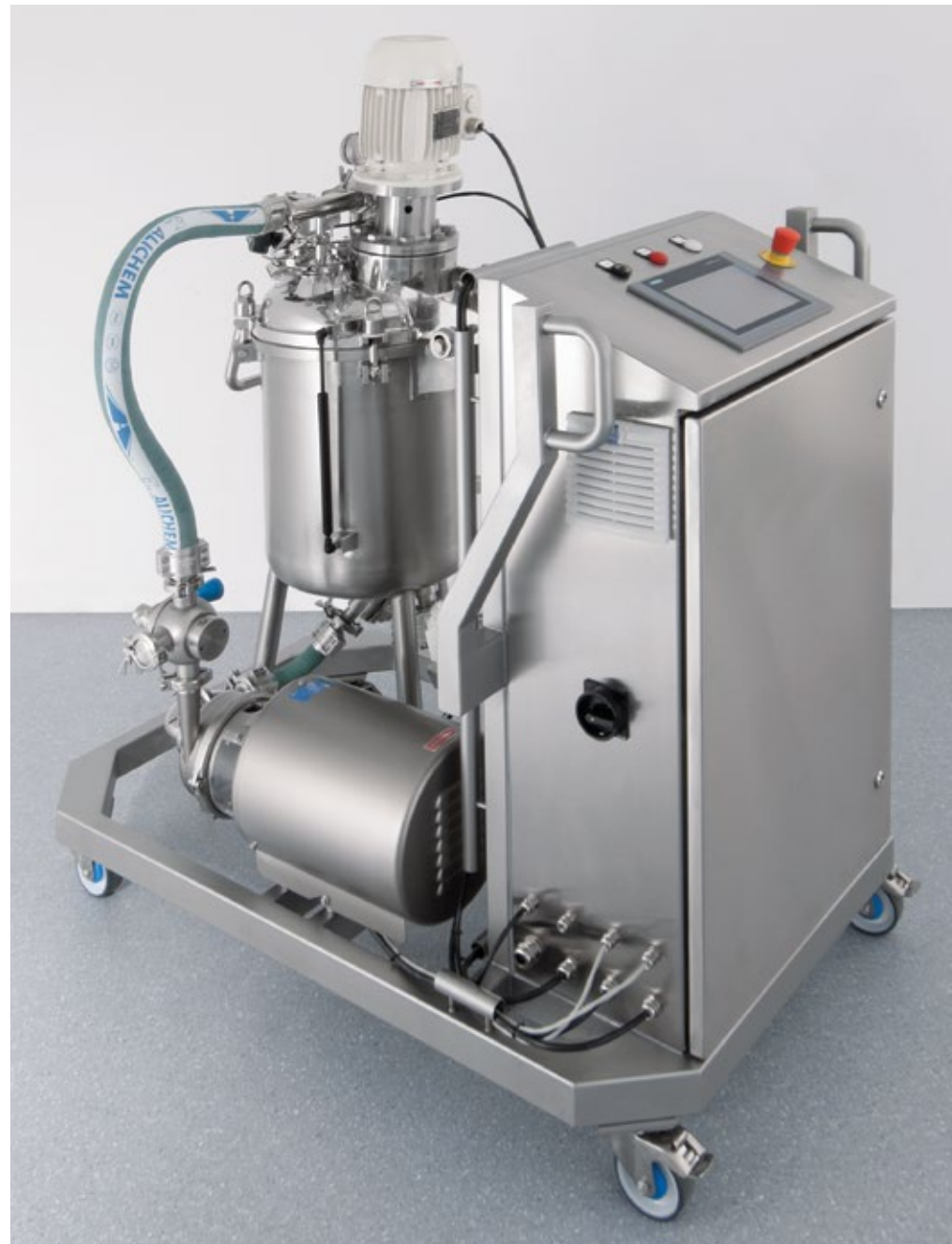
THEPROPREP Mobile auxiliary vessel for the preparation of solutions - 50 l (13 US gal) Client: Megapharma / Uruguay / 2014
