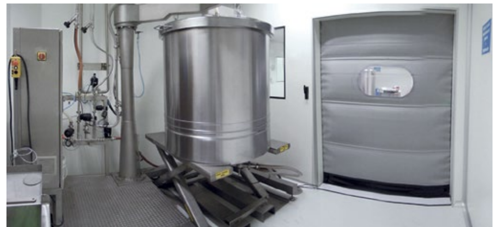
THEPROCLEAN Drying and CIP System with a tank. Client: Bayer / Venezuela / 2011
